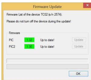
4. Click the enabled buttons "Update" if necessary, one after the other. The firmware is adapted automatically. The status will be displayed in the status bars.
