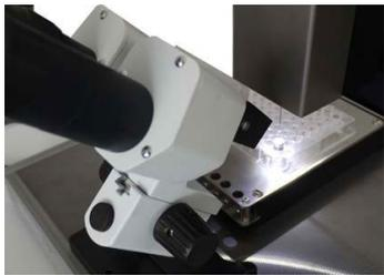
Move the z-axis and the carrier until the electrode tips approach the cross-hair by pressing the respective arrow keys. Alternatively, you may use the according buttons on the keyboard. Page up and page down keys for the z-axis and the four arrow key for the carrier. Fine tune the position until the alignment device is almost touched by the tip of the electrodes. If you do this the first time, you may have difficulties seeing the TEVC probe in three dimensions.
