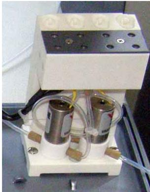
1. Connect the provided waste tubing to the waste outlet on the back of the rinse / transfer port station.
