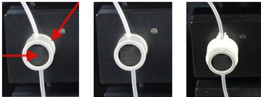
Twelve valves regulate the compound flow. Only one valve may be open at a time. Open a valve by hand or by a software command.
