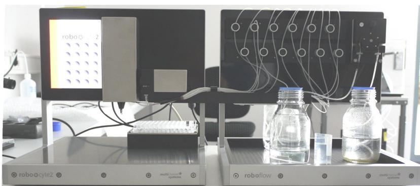
For high-throughput screens, the Roboocyte2 uses the advantages of an industry-standard liquid handler from Gilson (optional). The Gilson liquid handler version GX-271 is supported.
