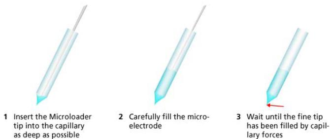
4. There should be no air bubbles in the glass capillaries. Otherwise, the electrode resistance will be too high. Gently tap on the glass to remove any air bubbles if necessary.
