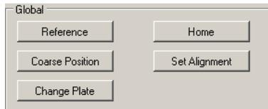
Click on the **"Reference"** button starts a reference movement of the z-axis and the well plate carrier. After performing a reference movement, the z-axis and the well plate carrier stops at a defined zero-position.
