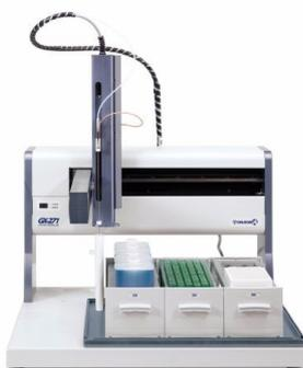
The use of the GX-271 liquid handler is an optional feature of the Roboocyte2. Test compounds are loaded onto the trays and aspirated by the Gilson probe. The liquid is transferred to the recording well via a peristaltic pump. A transfer port gives access to one or two larger medium bottles, for example for frog Ringer's or an often used reference compound.
