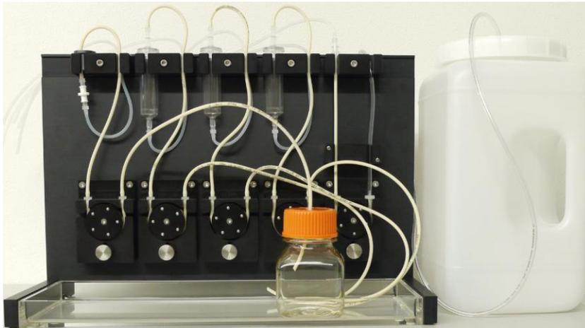
The **peristaltic pump PPS5 with software control** is developed for the perfusion of biological samples. The pumps are driven by stepper motors providing a very long lifetime without maintenance. The durable brushless motors are extremely reliable, show very constant rotation speed, are vibration free and have low electromagnetic emission. These characteristics make the PPS5-System an ideal choice for electrophysiological experiments.
