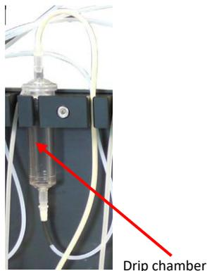
The drip chamber (droplet isolator) can be used to disrupt the direct liquid column from the pump to the sample. This can help to remove low frequency noise originating from the pulsation of the pump head. On the other hand, the droplet isolators make the flow speed inaccurate, and cause a continued flow even after the pump is stopped. If the flow rate is high (approximate  $> 6 - 8 \text{ ml / min}$ ) the droplet isolators will fill up over time and might even overflow.
