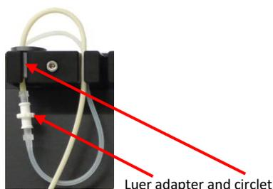
If you do not need the drip chamber, please use the circler and connect the heads of the tube with a luer adapter.
