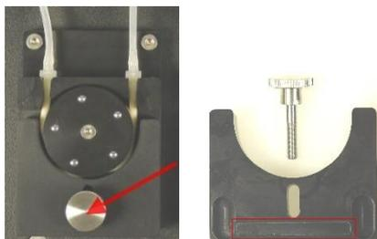
For connecting or changing the tubes, please open the screw and remove the bracket of the pump revolver. Insert the provided tube and fix it with the luer tube connectors in the denoted way. To remount the bracket, take care to insert the bar of the bracket into the corresponding socket on the pump housing. Fix the screw firmly.
