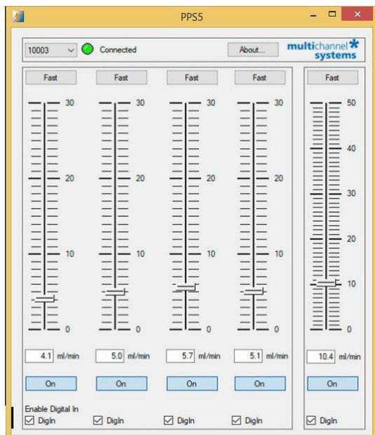
The intended use for the PPS5-System is the perfusion of a biological sample with different compounds and the aspiration of the overspill solution to the waste. To avoid flooding of the amplifier, the flow rate of the outlet must always be higher than the flow rate of the inlet.
