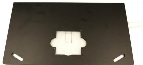
Turn the ground plate of the MEA2100 headstage around and put it onto a soft surface to avoid scratches. You need a TORX T6 screw driver to remove the designated screws (M2 x 4). Unscrew the six screws which fix the cover for the tubing. Keep the screws for reusing them later.
