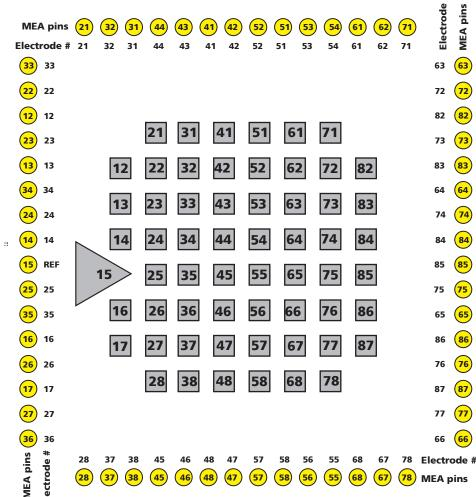
MEAs are not symmetrical! MEAs with internal reference electrode should be placed with reference electrode to the left side when looking directly to the opened amplifier.
