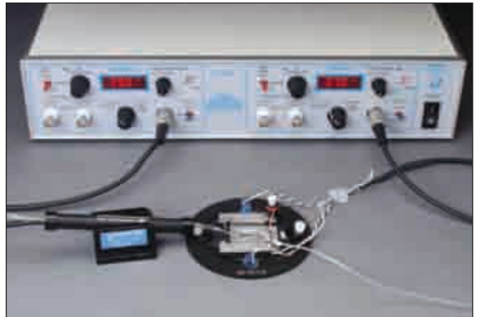
TC-344B – Dual Channel temperature controller shown with in-line solution heater and heated platform with connecting cable.
